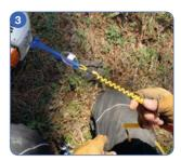
Connect the blue strap (1) around the rear attach of the chainsaw with a girth hitch.
